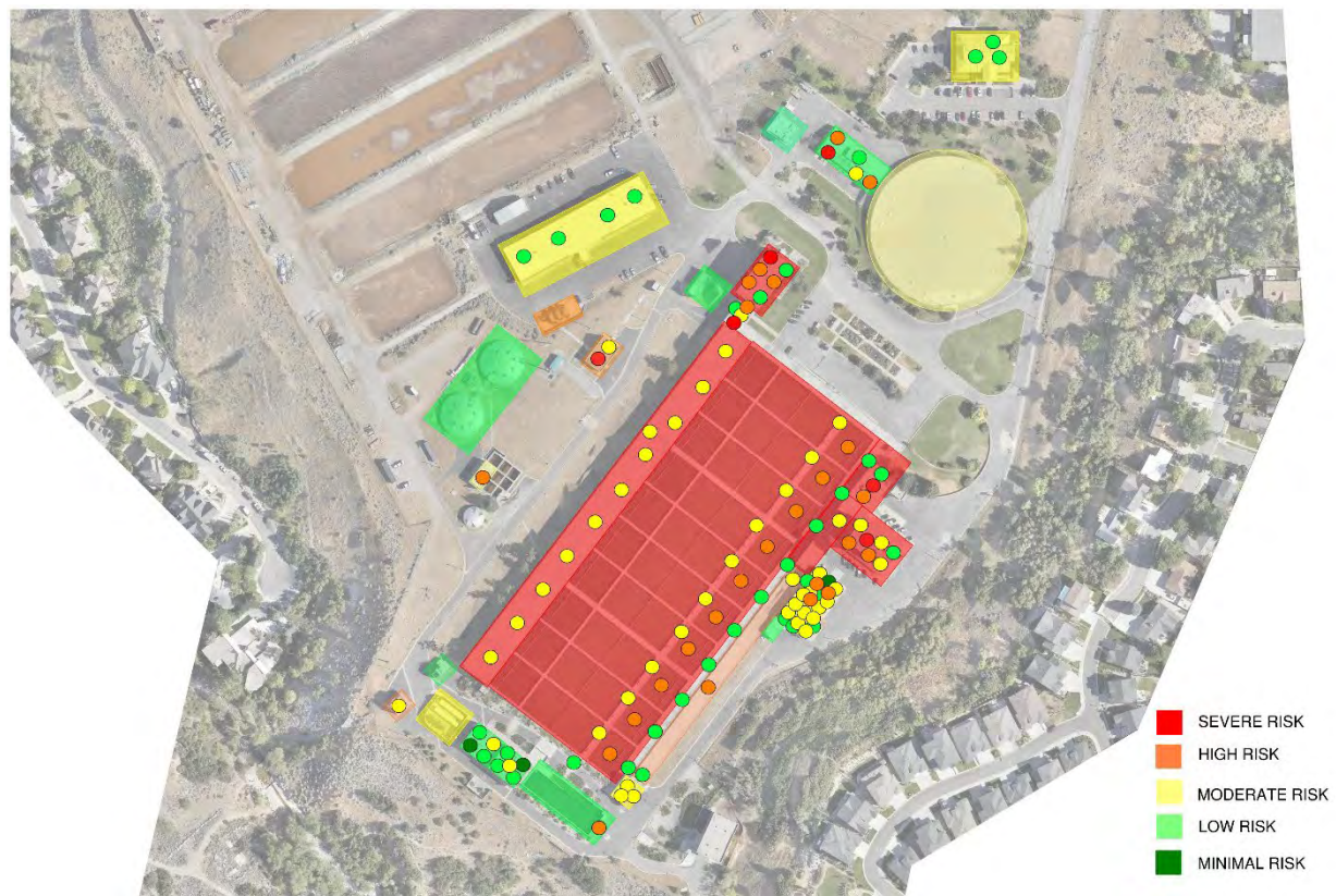
Figure 11. Building, Structure, and Component Group Risk Locations
